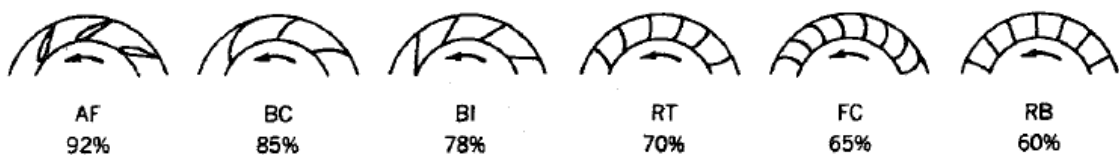
Figure 2-4: Schematic Representation of some Common Centrifugal Fan Blades in Descending Order (from Left to Right) of Their Approximate Maximum Efficiencies [7, Ch. 7, p. 7.2].
