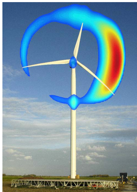
Figure 1: Wind turbine with projection of the noise source distribution in the rotor plane (averaged over many revolutions) (Oerlemans, 2011)
