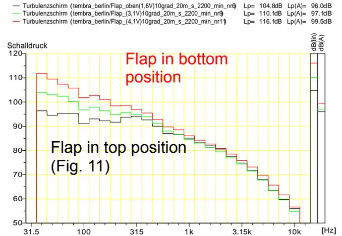
**Figure 12:** Sound pressure level reduction of the variable TEMBRA flap. Bottom, top and zero positions are shown, wind tunnel test at 20 m/s flow speed, angle of attack of the blade profile 10°.
