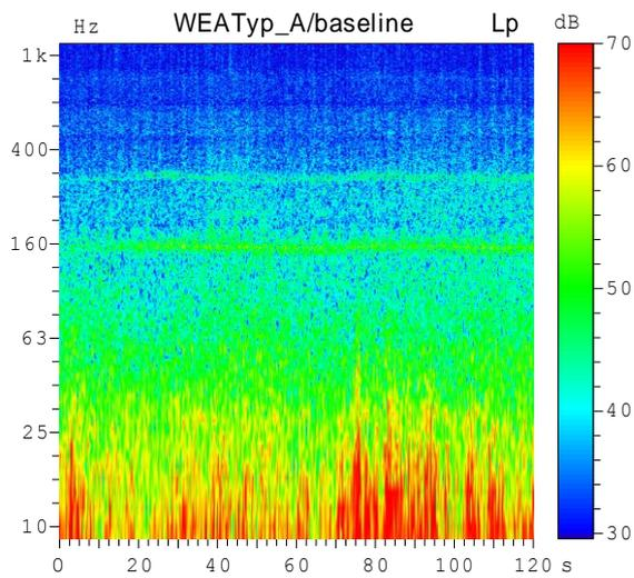
**Figure 5:** Sound pressure measurement of a 2MW wind turbine, noise occurs at app. 155 Hz and 310 Hz.
