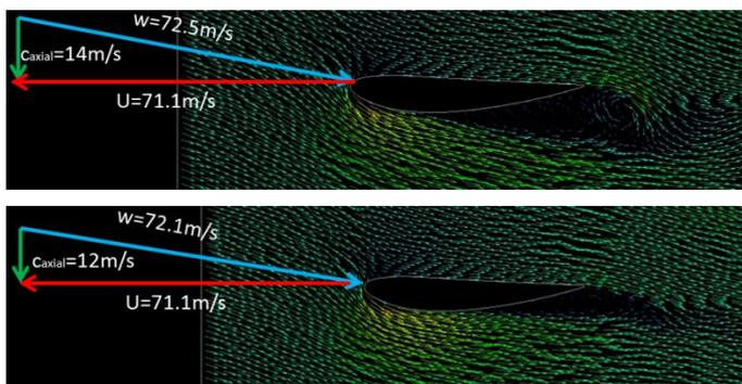
**Figure 7:** Inlet flow conditions on top and bottom positions of the blade generate different flow separation results,  $r/R=0.9$ ,  $n=28$  rpm.
