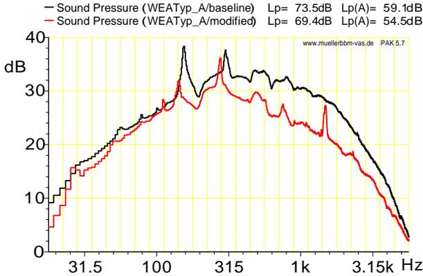
**Figure 10:** Sound pressure level reduction of app. 4 dB A-weighted overall level with optimised operating conditions (speed and pitch) on a 2 MW wind turbine
