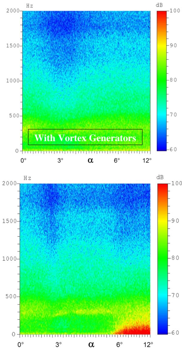
**Figure 14:** Sound pressure spectrogram with and without vortex generators, wind tunnel test, 20 m/s flow speed, angle of attack of the blade profile 0°.
