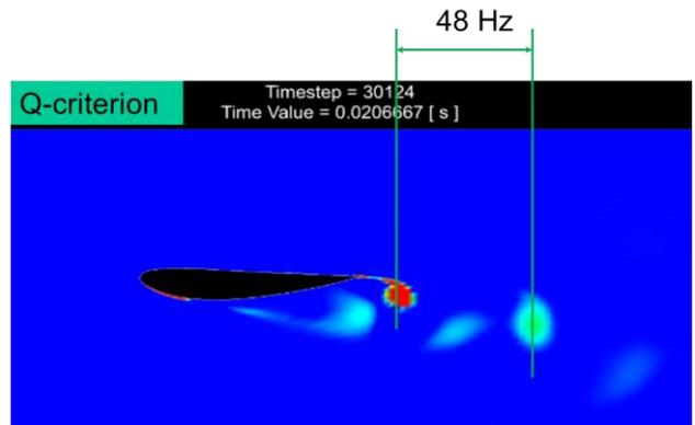
**Figure 8:** Unsteady CFD, 6 kHz sampling rate, Q-Criterion as a measure of loss, blade top position,  $r/R=0.9$ ,  $n=28$  rpm.
