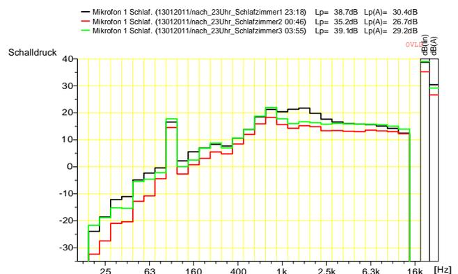
Figure 3: Example of sound pressure spectra with low frequency noise components (Here, the source mechanism is not a wind turbine!).
