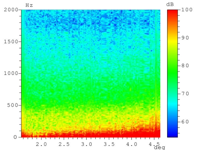
**Figure 13:** Sound pressure spectrogram of a TEMBRA flap variation from left=top position, shown in Fig. 11, to bottom position=right (4.5 deg), 20 m/s flow speed, angle of attack of the blade profile 0°.
