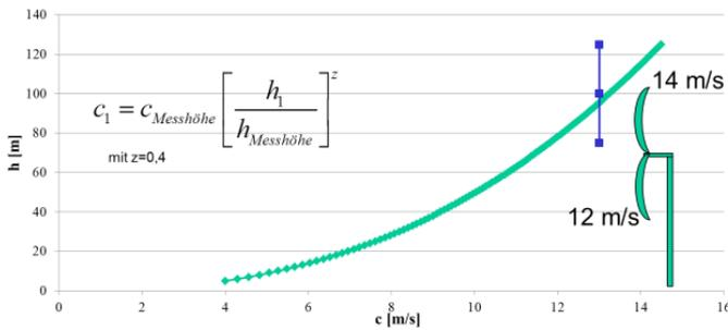
**Figure 6:** Atmospheric wind profile is responsible for different inflow conditions at the rotor blade at top (14m/s) or bottom positions (12 m/s).
