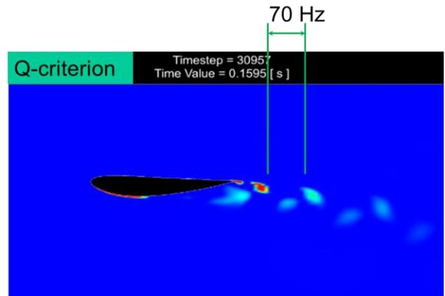
**Figure 9:** Unsteady CFD, 6 kHz sampling rate, Q-Criterion as a measure of loss, blade bottom position,  $r/R=0.9$ ,  $n=28$  rpm.
