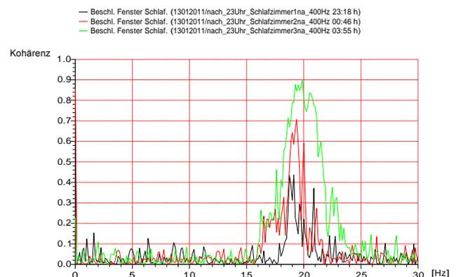
Figure 4: Coherence spectra of sound pressure and acceleration on the window pane show a relation to noise (Here, the source mechanism is not a wind turbine!).
