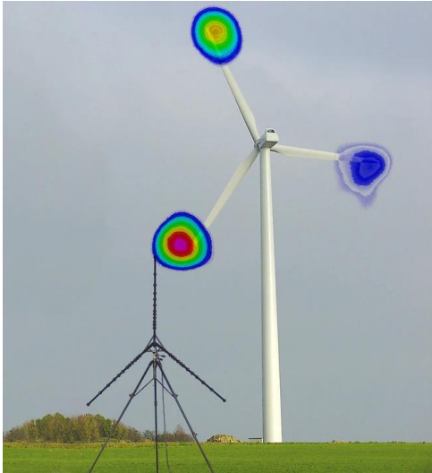
Figure 2: Measurement results known for some years by used beamforming methods, which show the blade tip as a main noise source for wind turbines.
