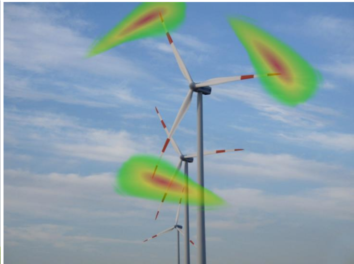
Figure 2: Measurement results known for some years by used beamforming methods, which show the blade tip as a main noise source for wind turbines.
